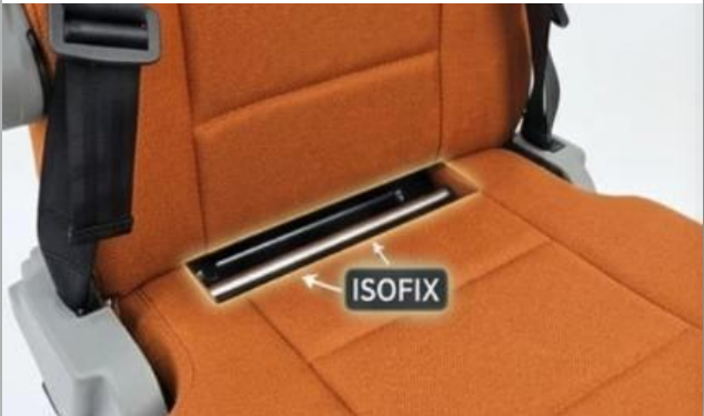
Step-1 To check ISOFIX connection points
